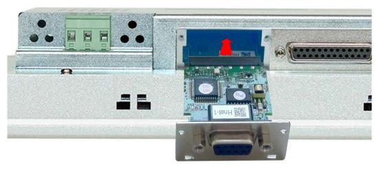
2. For installation insert the interface module into the opening. Push the interface module in the device until the holding plate fits to the housing. Here the interface module is put into the right position by 2 inner guide rails.
