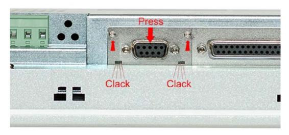
3. Now press the interface module downwards until the holding plate snaps into the lugs.
