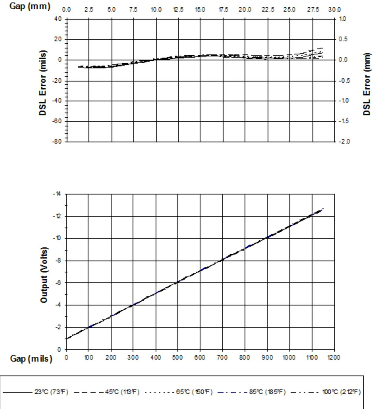
**Figure 8: Typical 3300 XL 50 mm 9 m Proximitors with 8 m of Extension Cable @ High Temperature (Probe is at 25°C.)**
