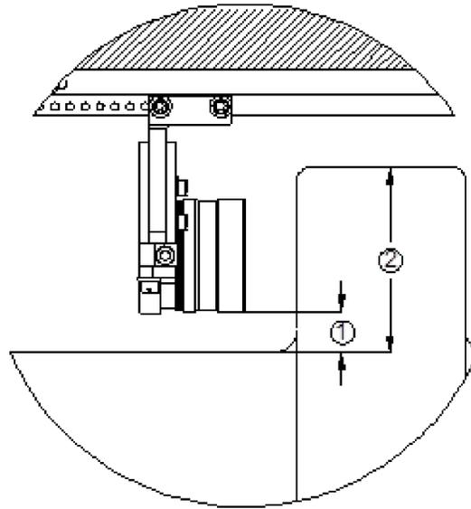
1. Shaft to side of probe distance.
