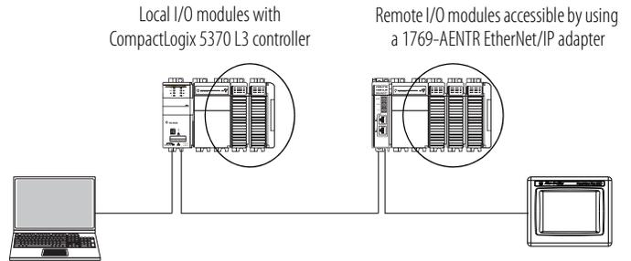
The modules mechanically lock together by means of a tongue-and-groove design and have an integrated communication bus that is connected from module to module by a moveable bus connector.
