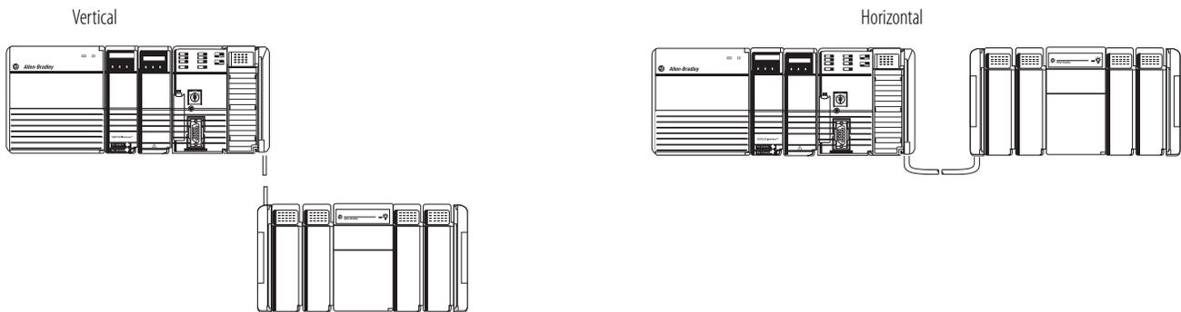
How you orient I/O banks determines the expansion cables you must connect the I/O banks.
