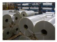
CP401 2-side sealable, containing no slip. Contains antiblock and antistat for processing purposes.
