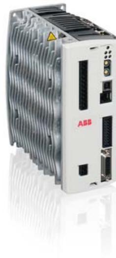
Compact motion control drive with real time Ethernet technology
