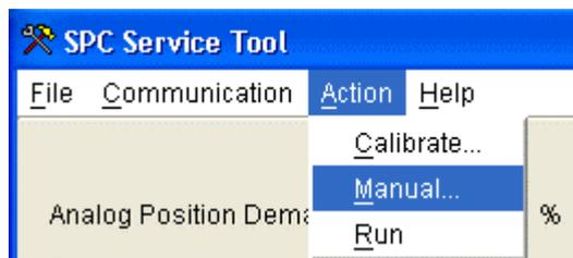
Figure 4-49. Selecting Manual Stroking
