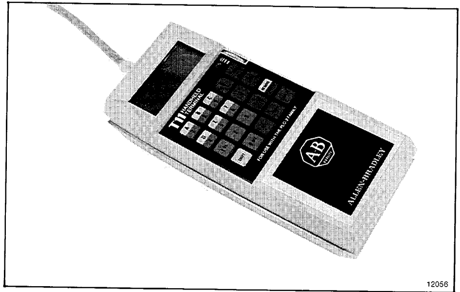
Figure 2.9 — Use the Hand Held Terminal to Access Data Table Information Stored in the Processor's Memory
