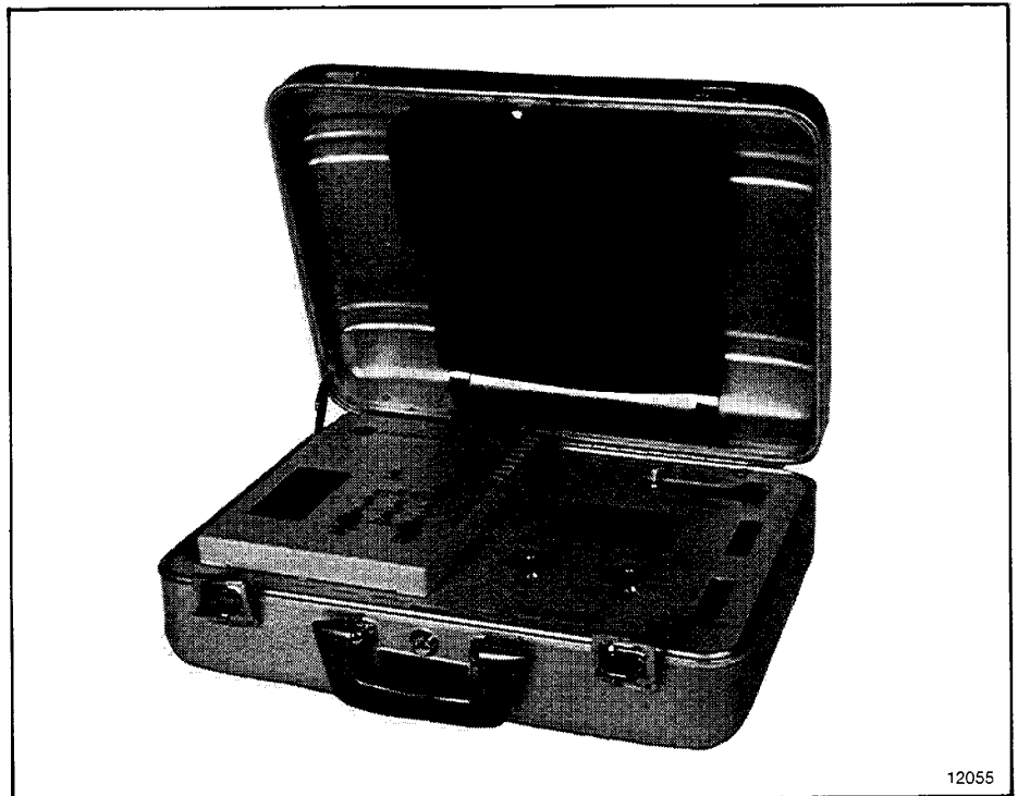
Figure 2.8 — Use the Data Cartridge Recorder to Record, Load and Verify the Processor's Total Memory
