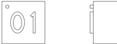
Figure 437 Node address jumper - front and side view
