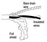
Twist the foil shield and drain wire together to form a single strand.
